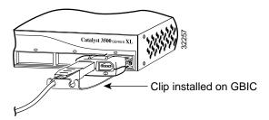
Step 5 Insert the GBIC into the slot. Follow the steps in the "Installing a GigaStack GBIC" section on page 2-4.
